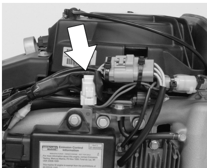
a- Fusible correct
