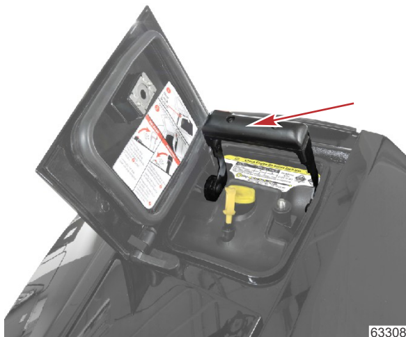
Handle locked in the lift position
