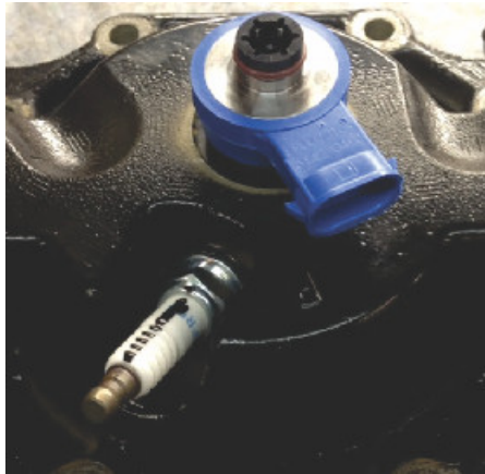
Example of an optimal aligned spark plug
