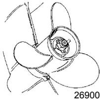
4. Place a block of wood between the gearcase and the propeller, and remove the propeller nut.
