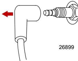
2. Remove the spark plugs. Replace the spark plug if the electrode is worn; the insulator is rough, cracked, broken, or blistered; or if the precious metal is not visible on the spark plug electrode.
