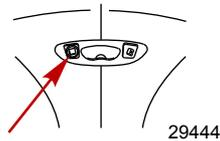
2. Attach a water hose to the fitting. Turn on the water and flush for 3–5 minutes.
