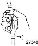
4. Set the lanyard stop switch to the "RUN" position. Refer to **General Information - Lanyard Stop Switch**.
