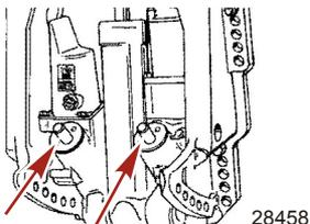
2. Lubricate the following with Extreme Grease or 2-4-C with PTFE.
