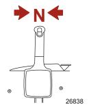
5. Move the throttle-only lever to the fully closed position or press the throttle-only button.
