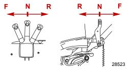
Remote control models - When shifting, always stop at the neutral position and allow the engine speed to return to idle.
