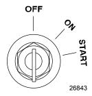
2. **Tiller handle models -** Reduce the engine speed and shift the outboard to neutral position. Push in the engine stop button or turn the ignition key to "OFF" position.
