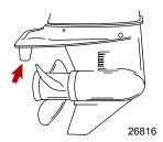
**NOTE:** Trim tab adjustment will have little effect reducing steering torque if the outboard is installed with the anti-ventilation plate approximately 50 mm (2 in.) or more above the boat bottom.
