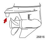
**NOTE:** Trim tab adjustment will have little effect reducing steering torque if the outboard is installed with the anti-ventilation plate approximately 50 mm (2 inches) or more above the boat bottom.
