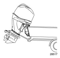
IMPORTANT: Do not rely on the power trim/tilt system or tilt support lever to maintain proper ground clearance for trailering. The outboard tilt support lever is not intended to support the outboard for trailering.
