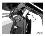
Remove the fill cap and check fluid level. The fluid level should be even with the bottom of the fill hole. Add Quicksilver or Mercury Precision Lubricants Power Trim and Steering Fluid. If not available, use automotive automatic transmission fluid (ATF).
