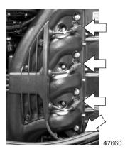
2. Remove the spark plugs to inspect.
