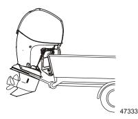
IMPORTANT: Do not rely on the power trim/tilt system or tilt support lever to maintain proper ground clearance for trailering. The outboard tilt support lever is not intended to support the outboard for trailering.
