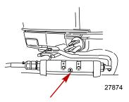
Steering Cable Grease Fitting (If equipped) - Rotate steering wheel to fully retract the steering cable end into the outboard tilt tube. Lubricate through fitting.
