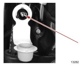
4. Push in on the fuel hose release tabs and disconnect the fuel hoses from the fuel filter.
