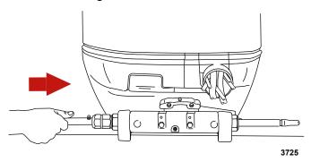
3. Tighten the nut to the specified torque.
