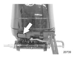
2. Pull down the rear cowl latch. Remove the top cowl.
