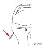
IMPORTANT: If no water is coming out of the water pump indicator hole, stop engine and check cooling water intake for obstruction. No obstruction may indicate a water pump failure or blockage in the cooling system. These conditions will cause the engine to overheat. Have the outboard checked by your dealer. Operating the engine while overheated will cause engine damage.
