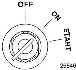
4. Within the first 10 seconds after the key switch has been turned on, move the remote control handle from neutral into forward gear 3 to 5 times. This will automatically start the priming process.
