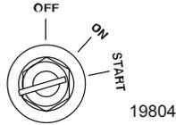
**NOTE:** The electronic starting system will automatically prime (choke) the engine and increase idle speed for starting.
