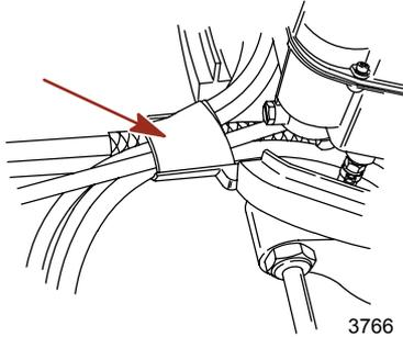
2. Fasten clamp together with two screws.
