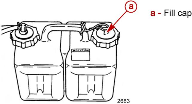
**IMPORTANT:** Do not remove the vent cap from the engine-mounted oil reservoir tank when filling the tank. Removal of the vent cap may damage the threads in the oil reservoir tank. Damaged threads may result in future oil leakage.
