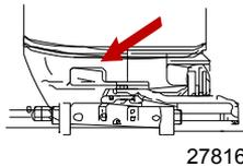
2. Lift up the rear cowl latch. Remove the top cowl.
