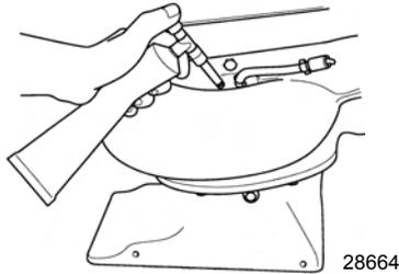
2. Open the fuel tank vent screw, located in the filler cap, on manual venting type fuel tanks.
