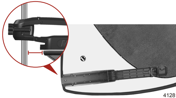
Mount on deck with a 3 in. clearance
