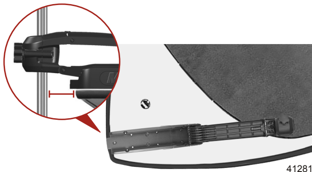
Mount on deck with a 3 in. clearance
