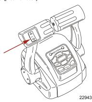
Neutral lights - The neutral lights illuminate when the engine is in neutral gear position. The lights will flash when the engine is in throttle only mode.
