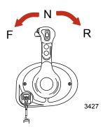
• When shifting, always stop at neutral position and allow the engine speed to return to idle.
