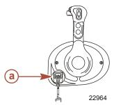
7. Control handle tension adjustment screw - This screw can be adjusted to increase or decrease the tension on the control handle (cover must be removed). This will help prevent unwanted motion of the handle in rough water. Turn screw clockwise to increase tension and counterclockwise to decrease tension. Adjust to tension desired.
