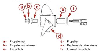
7. Place a block of wood between gearcase and propeller and torque to specifications.
