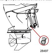
NOTE: The manual tilt release valve must be tightened before operating the outboard to prevent the outboard from tilting up during reverse operation.
