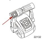
Neutral lights - The neutral lights illuminate when the engine is in neutral gear position. The lights will flash when the engine is in throttle only mode.
