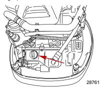
IMPORTANT: Inspect oil for signs of contamination. Oil contaminated with water will have a milky color to it; oil contaminated with fuel will have a strong fuel smell. If contaminated oil is noticed, have the engine checked by your dealer.
