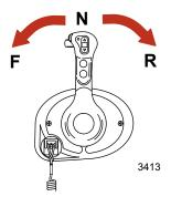
2. Shift lock - Pressing the shift lock allows the engine to shift. The shift lock must always be pressed when moving the control handle out of the neutral position.
