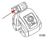
3. Control handle tension adjustment screw - This screw can be adjusted to increase or decrease the tension on the control handle (cover must be removed). This will help prevent unwanted motion of the remote control handle in rough water. Turn the screw clockwise to increase tension and counterclockwise to decrease tension. Adjust to the desired tension.
