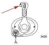
3. Trim switch (if equipped) - Pressing the trim switch allows the engine to trim up or down.
