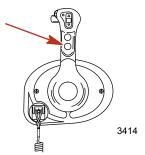
6. Lanyard stop switch - Turns the ignition off whenever the operator (when attached to the lanyard) moves far enough away from the operator's position to activate the switch.
