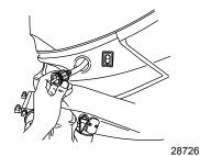
3. Thread a water hose into the flush fitting.
