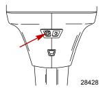
2. Attach a water hose to the fitting. Turn on the water and flush for 3 to 5 minutes.
