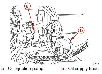
IMPORTANT: Fill the engine fuel system with fuel before priming the oil injection pump. Otherwise, the fuel pump will run without fuel during the priming process and may be damaged.
