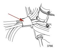
2. Fasten clamp together with two screws.
