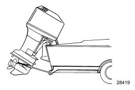
IMPORTANT: Do not rely on the power trim/tilt system or tilt support lever to maintain proper ground clearance for trailering. The outboard tilt support lever is not intended to support the outboard for trailering.
