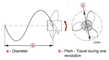
The following are some propeller basics that will help you determine the correct propeller for your boating application.
