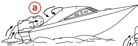
a- Running the boat with the trim angle of the bow too high.
