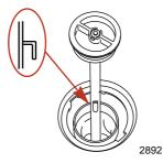
5. Slowly fill the oil tank with the specified oil. Do not overfill. Add only enough oil to bring the oil level up to the bottom of the fill neck.
