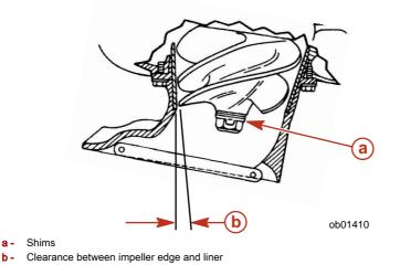
Check the impeller clearance by sliding a feeler gauge through the intake grate and measure the clearance between the impeller edge and liner. If adjustment is required, refer to **Impeller Removal and Installation.**
