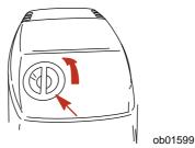
2. Remove oil filler cap and pull out dipstick.
