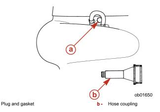
3. Attach a water hose to the hose coupling. Slowly turn on water. Start the engine and run it at idle speed only.
