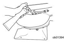
2. Open fuel tank vent screw (in filler cap) on manual venting type fuel tanks.
