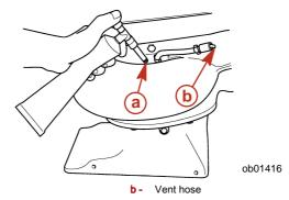
iii. Reconnect the vent hose onto the grease fitting after greasing.
