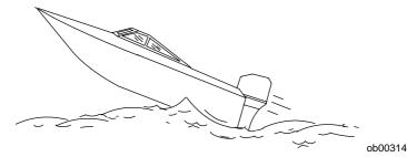
The primary concern is the boat changing direction while in the midst of the jump. In such case the landing may cause the boat to veer violently in a new direction. Such a sharp change in direction can cause occupants to be thrown out of their seats, or out of the boat.
