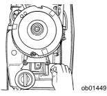
6. If engine is cold, hold the fuel primer button in and pump up the fuel pressure with the fuel primer bulb.
