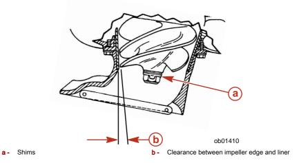
6. After setting the impeller height, tighten the impeller nut snug with a wrench. Secure impeller nut by bending tabs against the flat on the impeller nut.
