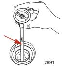
4. Hook the dipstick on the tank during filling.
