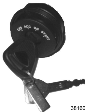
Four position key switch
