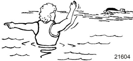
Always slow down and exercise extreme caution any time you are boating in an area where there might be people in the water. Whenever a boat is moving (even coasting) and the gear shift is in neutral, there is sufficient force by the water on the propeller to cause the propeller to rotate. This neutral propeller rotation can cause serious injury.
