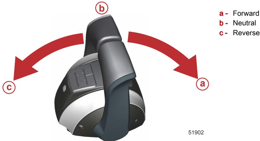
The amount of force needed to move the handles and to move the handles through the detents is adjustable to help prevent unwanted motion.
