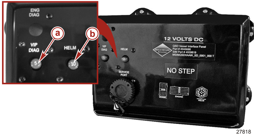
Vessel Integration Panel (VIP) circuit breakers
