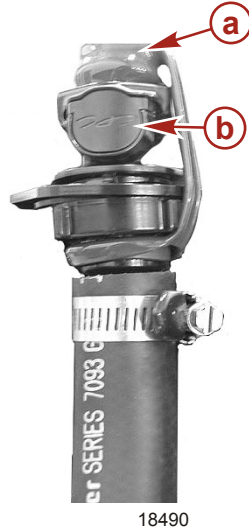
Dust cover installed in the flush socket
