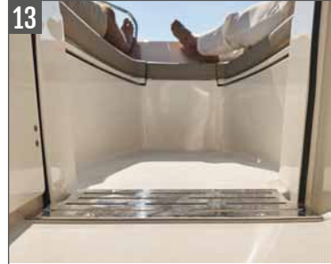
Unique bow drain system avoids water to accumulate and flow into the cockpit
