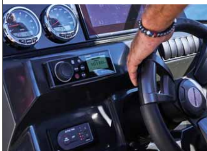
Stylish windshield and ergonomic helm station with instrumentation and mounting space for a 9" GPS/Chart plotter. Integrated armrests and cup holder
