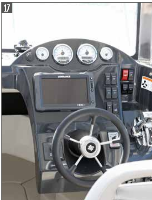
Integrated helm with hydraulic steering, SmartCraft instrumentation, mounting area for 9" GPS/Chart plotter and stereo
