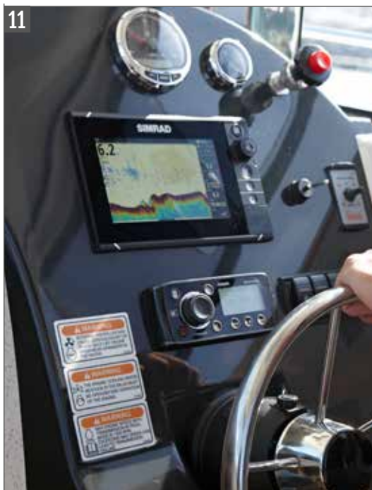
Integrated helm with hydraulic steering, SmartCraft instrumentation and 7" GPS/Chart plotter
