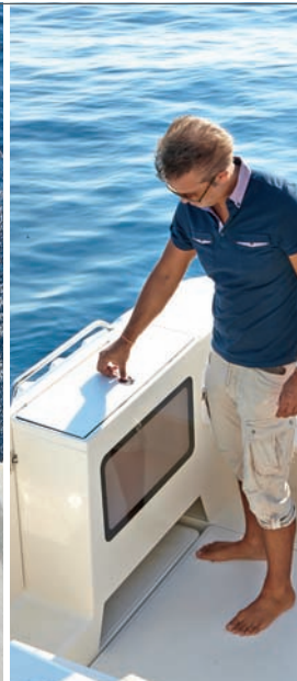
4 Livewell system with bait preparation station & raw water wash down
