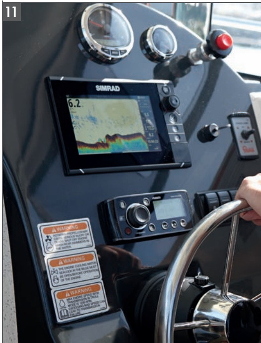
Integrated helm with hydraulic steering, SmartCraft instrumentation and optional 7" GPS and Bluetooth radio
