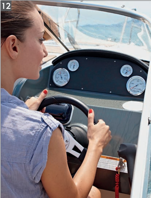
Integrated helm with hydraulic steering, SmartCraft instrumentation, mounting area for optional 7" GPS/depth sounder and 12v outlet
