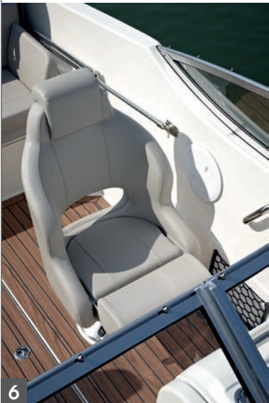
Pilot and co-pilot seats with flip bolster and swivel to ensure driving comfort
