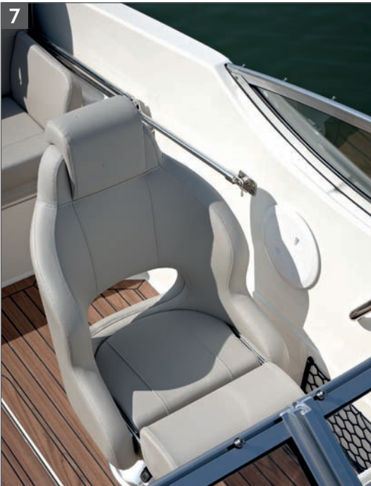
7 Pilot and co-pilot seats with flip bolster and swivel to ensure driving comfort
