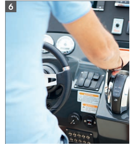
6 Ergonomic helm with instrumentation, optional 9" Simrad chartplotter, vessel view and smart craft instrumentation
