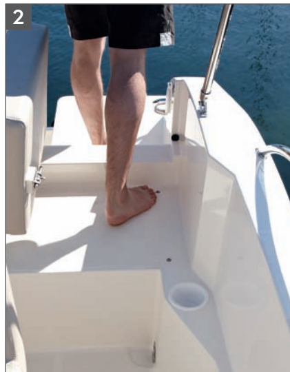
2 Unobstructed access from the swimming platform to the cockpit thanks to the pivoting backrest
