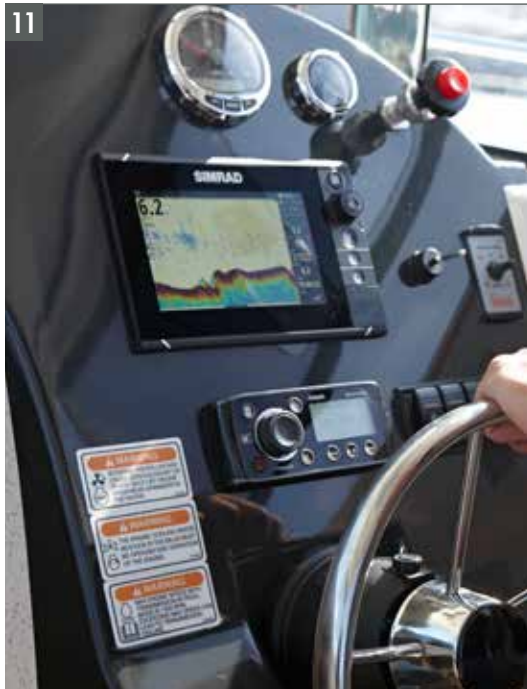
Integrated helm with hydraulic steering, SmartCraft instrumentation and optional 9" GPS and Bluetooth radio
