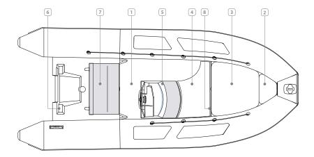
1 Optimized deck to ensure easy onboard movement; deep deck for child safety
