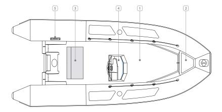
1 Largest and basic deck plan to ensure easy onboard movement; deep deck for child safety
