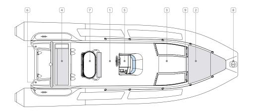
1 Optimized deck to ensure easy onboard movement around the console, leaning post and seats
