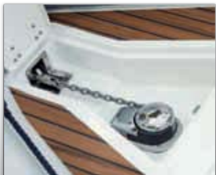
Electric windlass with anchor (optional)
