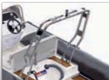
Folding navigation frame S-5/6/7 with navigation lights
