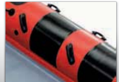
Tube reinforcement and handles (diver)
