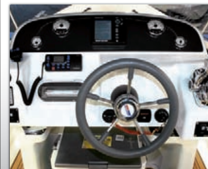
Dashboard with Northstar 657 combined sounder/GPS (standard)
