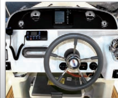
Dashboard with Northstar 657 combined sounder/GPS (optional)
