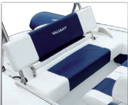
Folding stern seat (doubles the surface of the sundeck in horizontal position)
