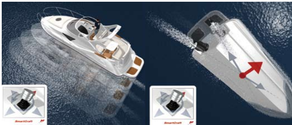
Axius' individual drives simultaneously thrust in forward and reverse to direct the boat.
