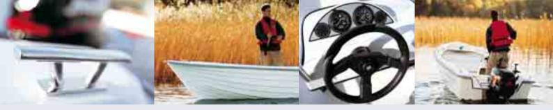
The A46 is built in the finest Uttern tradition, with a sturdy cockpit and windscreen. The boat is supremely practical and reliable with its self-bailing deck, wide clinker-built hull, high freeboard and a solid keel giving it extra stability. There is ample loading room and increased stowage in dry storage lockers under the aft and mid bench-seats. You can cover long distances in the Uttern A46 and moor it almost anywhere. And on top of that, it functions well as a rowing boat.
