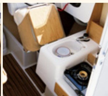
635 Weekend. The compact galley includes a freshwater-supplied sink hidden under the skipper's seat.
