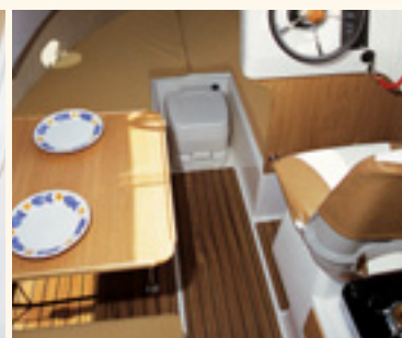
635 Weekend. Space on board has been maximised and the portable head is neatly secured between the forward V-berths.
