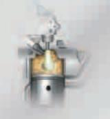
Unlike other direct injection systems, OptiMax uses an exclusive twostage process. A burst of air at 80psi shoots through the fuel, breaking it into a fine mist. This mist creates more surface area for combustion and stays in the cylinder longer, resulting in a more consistent and complete burn.
