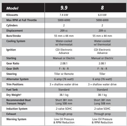
Dry weight specification is for lightest version model and excludes engine oil, rigging, hardware and propeller.
